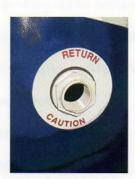
12 Slide the threaded portion of the wall fittings (2) through the openings marked "Suction" and "Return" from the inside of the pool. Firmly tighten the lock nut from the outside of the liner until the wall fitting is firmly seated on both sides of the liner.
