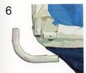
Each corner opening should now have the ends of two Top Rails exposed, one male and one female.
